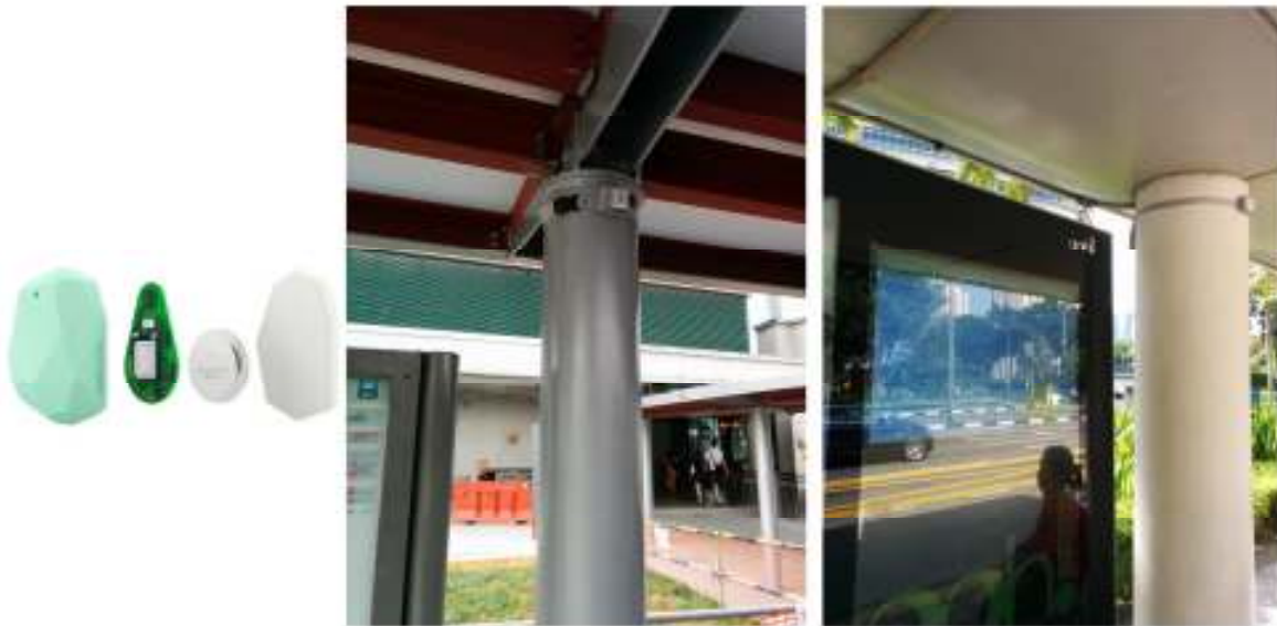
FIGURE 2 Left: Estimote iBeacon used in the study; Middle and right: iBeacon installation at two bus stops.
